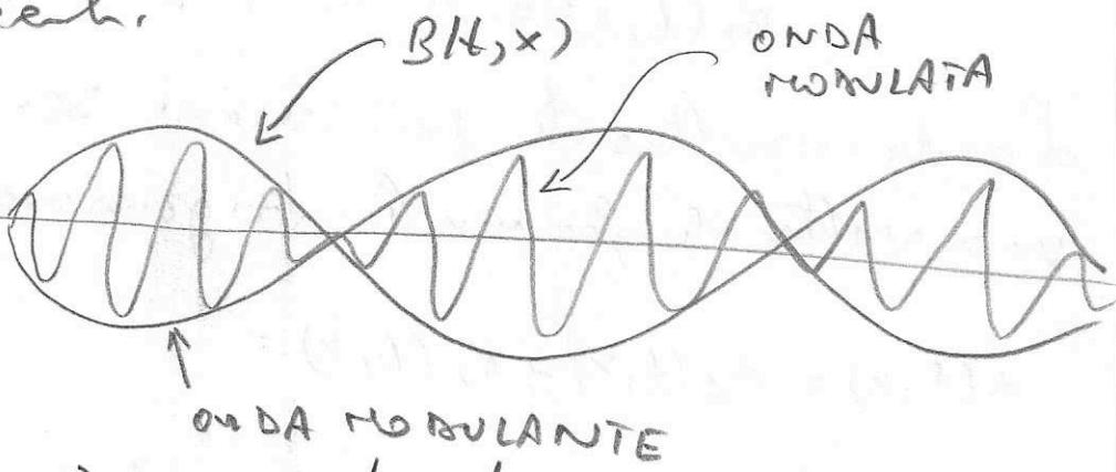
$$v_B = \frac{\omega_1 - \omega_2}{\omega_1 - \omega_2} = \frac{w_1 v - w_2 v}{w_1 - w_2} = \frac{(w_1 - w_2)v}{w_1 - w_2} = v$$
