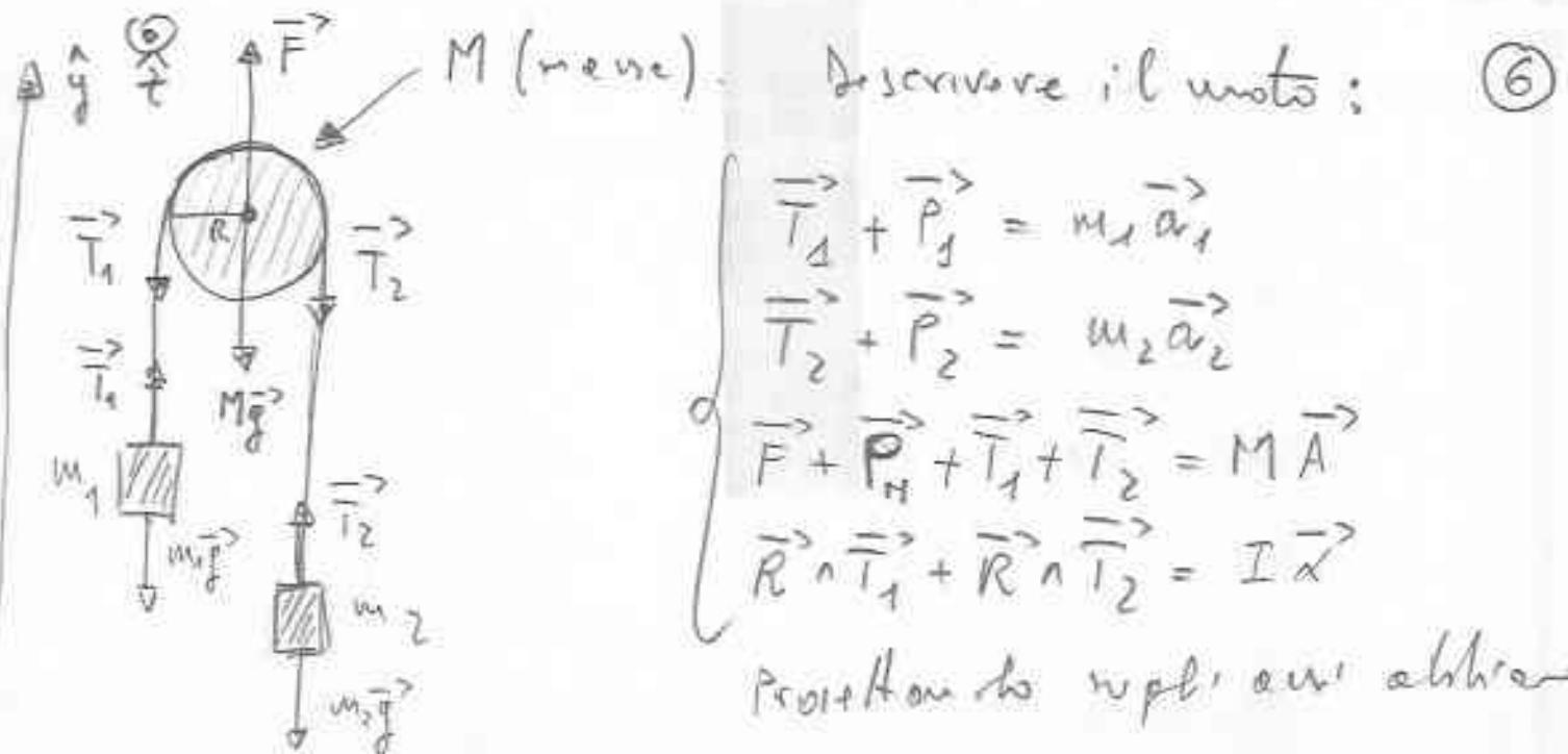
$$\left\{ \begin{array}{l} \vec{T}_1 + \vec{P}_1 = M_1 \vec{a}_1 \\ \vec{T}_2 + \vec{P}_2 = M_2 \vec{a}_2 \\ \vec{F} + \vec{P}_N + \vec{T}_1 + \vec{T}_2 = M \vec{A} \\ \vec{R} \wedge \vec{T}_1 + \vec{R} \wedge \vec{T}_2 = I \vec{\alpha} \end{array} \right.$$
