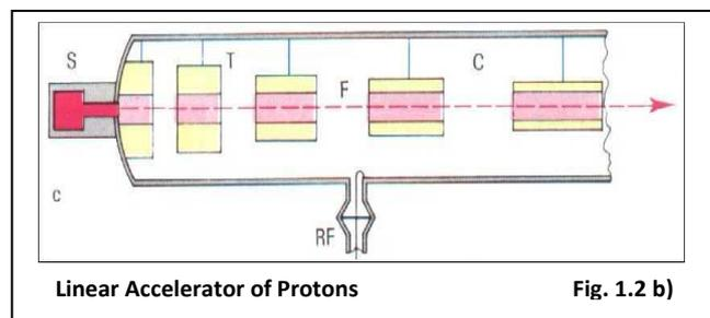
**Fig. 1.2 b)** It's composed of a resonant cavity excited by a radio-frequency oscillator. The synchronism between the electric field and the particle, occurs by introducing in the cavity several cylinders that have increasing length and decreasing diameter. In this way, the protons are always in synchronism with the electric field so one has always acceleration. These machines are used to inject particles in the proto-synchrotrons.
