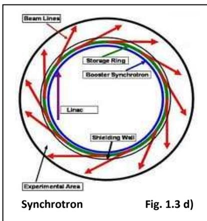
**Fig. 1.3 d)** It's an accelerator of electrons (electro-synchrotron) or protons (proto-synchrotron) based on the principle of phase stability. Particles are supported on a circular orbit in synchronism with the accelerating electric field. They have annular magnet frequency modulation of electric field and periodic modulation of magnetic field. Energies reached: 1 TeV.
