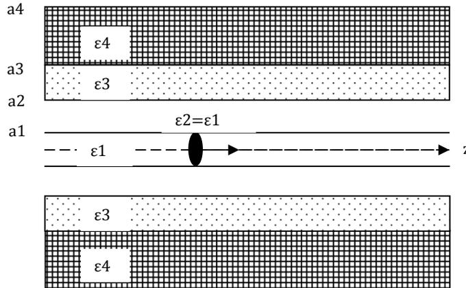
**Fig. 4.2** A relativistic plane disk of radius  $a_1$ , total charge  $Q$  and charge transverse distribution  $\rho(r, \vartheta)$  moving with velocity  $v \sim c$  along the  $z$ -axis of uniform, circular cylindrical two-layer tube of inner radius  $a_2 = b$ . The disk center coincides with the tube axis. The boundary between two layers is located at  $r = a_3$  and the outer radius of the tube is  $a_4$ . Outside the tube is vacuum and the layer can be either dielectrics or metals.
