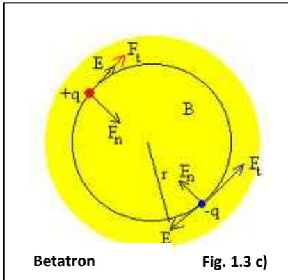
**Fig. 1.3 c)** It's an accelerator of electrons that acts as a transformer: the primary is composed of an envelopment and the secondary is composed of a beam of electrons. Electrons are supported on a circular orbit by the magnetic field and they are accelerated by the induced electric field. The beam is deviated from the orbit and it's directed towards a target. Energies reached: 350 MeV.
