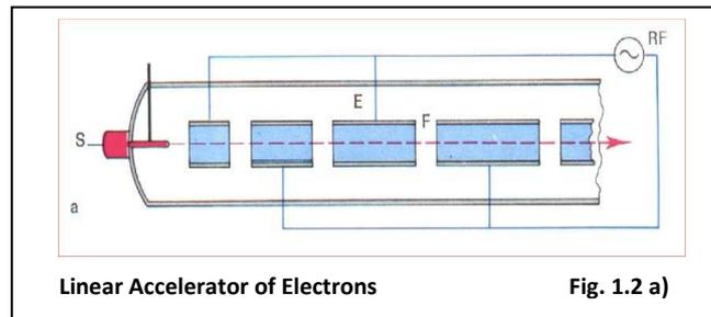
**Fig. 1.2 a)** Each section is composed of a wave guide, in the shape of cylindrical conductor, fed by a radio-frequency generator. Inside there are several conducting drift tubes through which the beam moves. Electrons, injected by an electrostatic accelerator at the speed of light, travel in phase with electromagnetic wave in the same direction, and they are always accelerated by the electric field. Under these assumptions the principle of phase stability is enforced.
