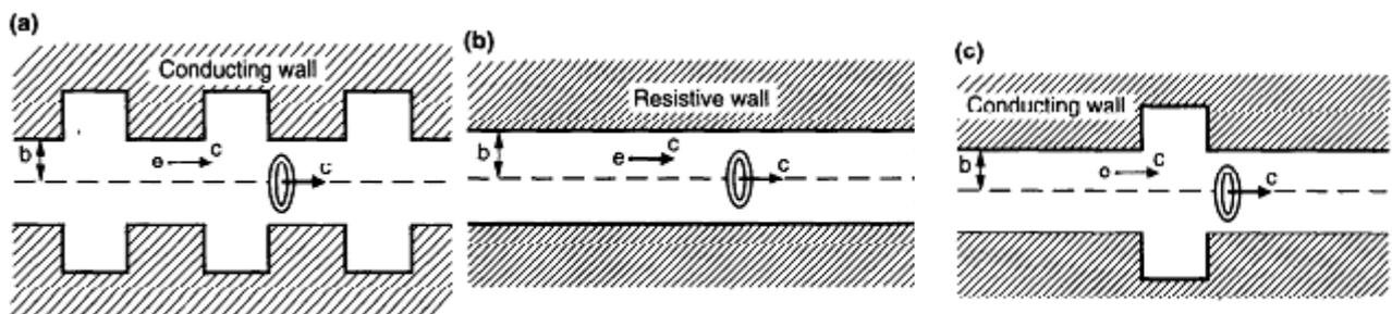
**Fig. 2.1** Examples of vacuum chamber pipe that generates wake fields. **(a)** Case of periodic structure. **(b)** Case of resistive wall. **(c)** Case of single structure.
