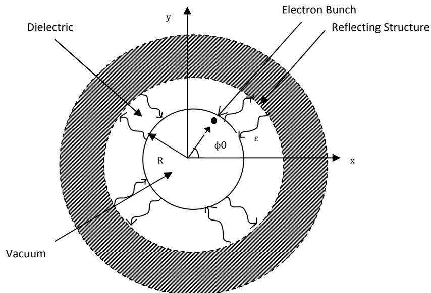
**Fig. 4.3** A point charge  $q$  located at  $r = r_0$  and  $\phi = \phi_0$  moves parallel to the  $z$ -axis at a velocity  $v$  in a vacuum tunnel of radius  $R$ . The latter is surrounded by a dielectric structure that confines the electromagnetic mode.
