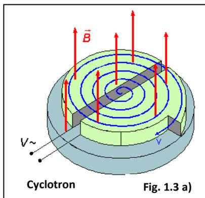
**Fig. 1.3 a)** It's composed of a circular cavity where there are two copper electrodes, in the shape of  $D$ , that are connected to the voltage radio-frequency generator. Ions describe spiral trajectories and, going out from the first electrode, they suffer the action of the electric field, which accelerates them towards the second electrode. After going along a semicircle they appear and they are accelerated by the electric field. Energies reached: 20-25 MeV.
