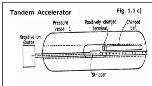
**Fig. 1.1 c)** It's a type of Van de Graaff accelerator with two phases. In the first one, protons are changed in  $H^-$  ions so they are accelerated by the electric field that exists between the source to earth and the high voltage electrode. Ions  $H^-$  are changed in ions  $H^+$  which are accelerated towards the target to earth in the second phase.
