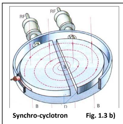
**Fig. 1.3 b)** This type of accelerator is used to accelerate protons in the energy relativistic region: in a range of energy until  $200 \text{ MeV}$  for nuclear studies and until  $700 \text{ MeV}$  for the production of mesons and their interactions. The rotation frequency depends on the energy. According to the principle of phase stability, the phase synchronism occurs by decreasing the frequency of oscillator.
