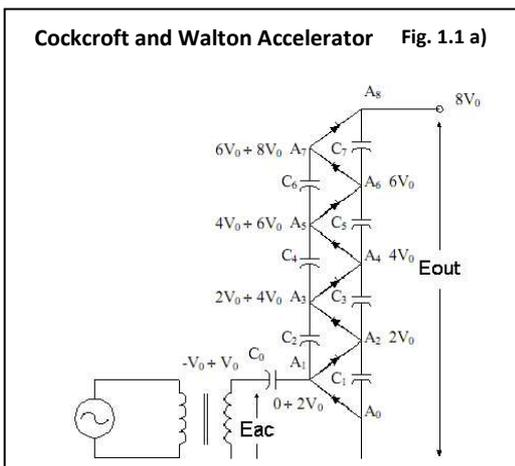
**Fig. 1.1 a)** Its main characteristic is the high voltage generator based on a voltage multiplying circuit which consists of two columns of capacitors in series connected to several diodes in series. A column is connected to the secondary of a transformer and the second one has an extremity to earth and another one is brought to an high direct voltage. The maximum energy reached is 2 MeV.
